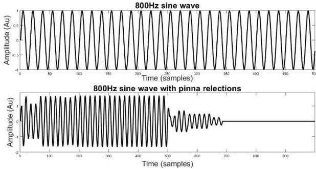
Figure 4- 800Hz sinewave before and after pinna reflections for a 0° elevation are applied.
