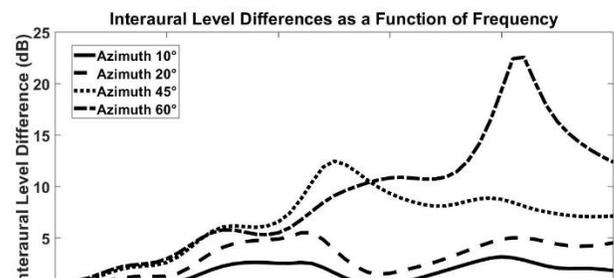
Figure 1- Simulated ILD data as a function of frequency.
